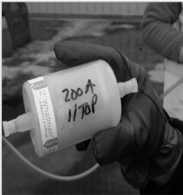
A Hepa Cap 75 filter which holds approximately 50 g of sample"
